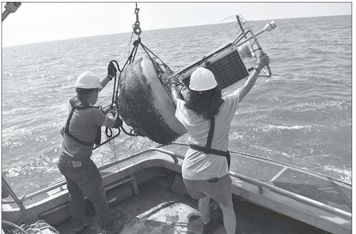
Researchers from the Cooperative Institute for Great Lakes Research lift a water monitoring buoy out of Lake Erie. Photo by Ray Garcia, CNS.
