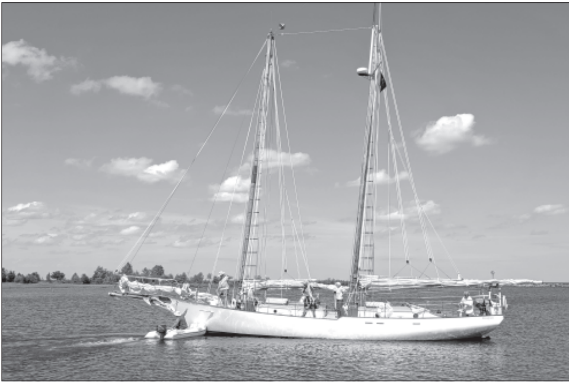
Perception also visits Harrisville Harbor overnight. This 68-foot steel-hulled schooner was built in 1985 from plans designed by the famous naval architect L. Francis Herreshoff. Perception is gaff-rigged, and her masts stand 70 feet tall. Owned by Michigan Challenge Traditional Sail Training, she is homeported out of Northport, Mich. Photo courtesy of Jim Ferguson.
