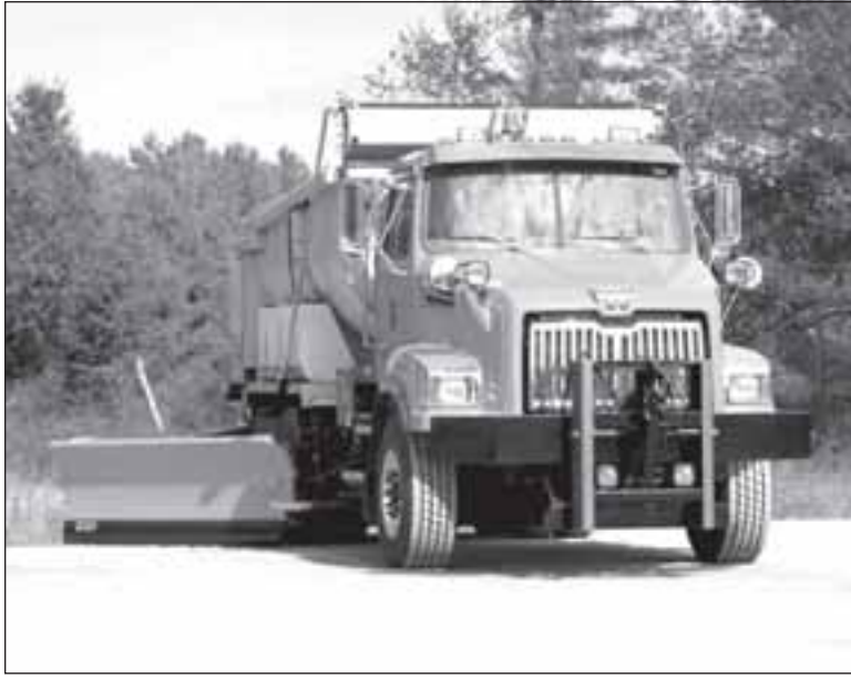
One of the three new tandem plow trucks with a wing plow attachment that the Alcona County Road Commission will be using this winter. Courtesy photo.
