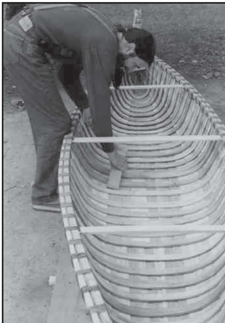
Curved ribs made of white cedar are added to the full length of the canoe to provide support and shape. Photo courtesy of Eric Mase.
