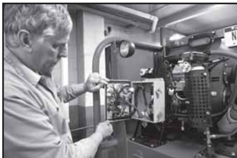
DNR heavy equipment mechanic Mike Pickler completes electrical circuits for a fire engine that will be used in wildfire suppression efforts.
