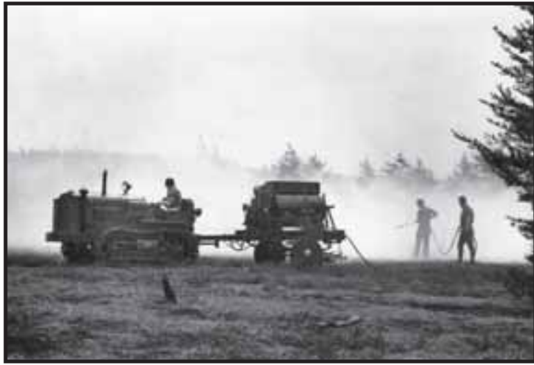
This historical photo shows a pull-behind water unit connected to hand lines for fire suppression. Photo courtesy of Michigan DNR.
